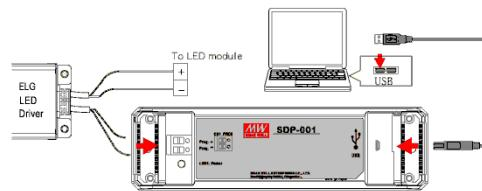
The D2 option provides user programmable dimming over time in 4 stages. This allows reduced energy/ carbon footprint and longer LED life for street lighting. Contact us for details.
